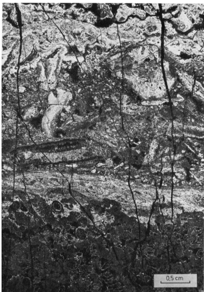
Fig.6. Typical dolomitization-lithification-reworking sequence: biodismicrite with dolomite-lined shrinkage pores at the base covered by a faintly laminar dolomite crust (white) and its reworking products in a calcite matrix (gray). The top of the specimen is a dolomitic stromatolite layer with calcite-filled shrinkage voids (black). Negative print of an acetate peel.
